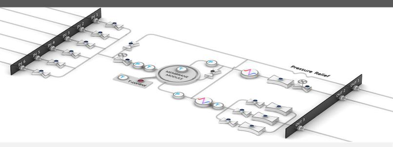
The Convergence Gas Booster has been developed to boost inlet gases to a higher pressure. The system is equiped with an air driven pump and can boost gases to the user defined setpoint.
